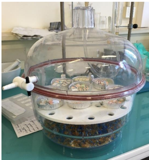
Figure 2.26 Reservation of the drying specimens
